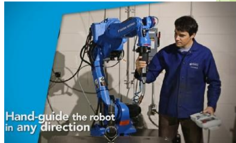
Robot with Kinetic Teaching for Limpad welding MA1440
