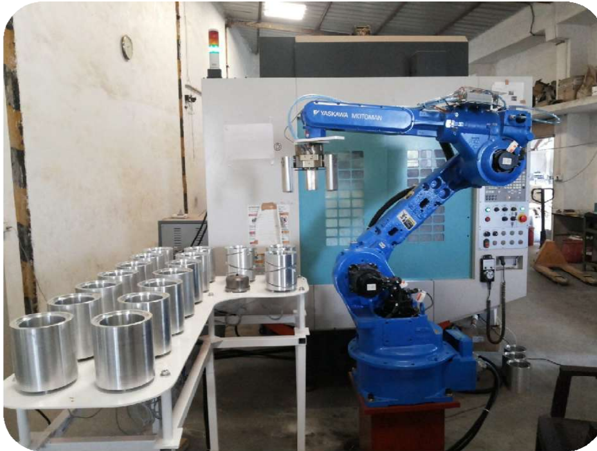
Machine Trending– Pick & Place with robotic system integrated with three machine
