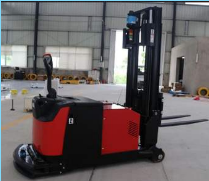
AGV with Counter balance for Heavy Load 2.5 T
